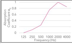
Sonaslat fixed over 50x50mm timber battens and Maxi Slab 50 infill (Ref: 05792-6277):
